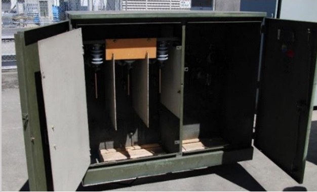
Specimen 1 6kA, 40 cycles, 7.4 cal/cm 2
