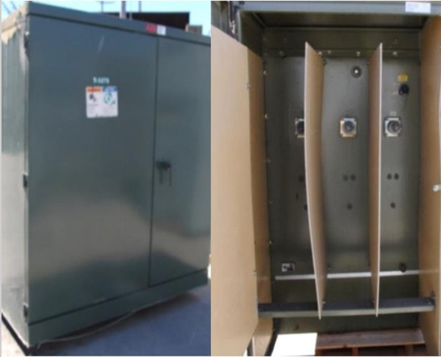
Specimen 5 3kA, 40 cycles, 9.2 cal/cm 2
